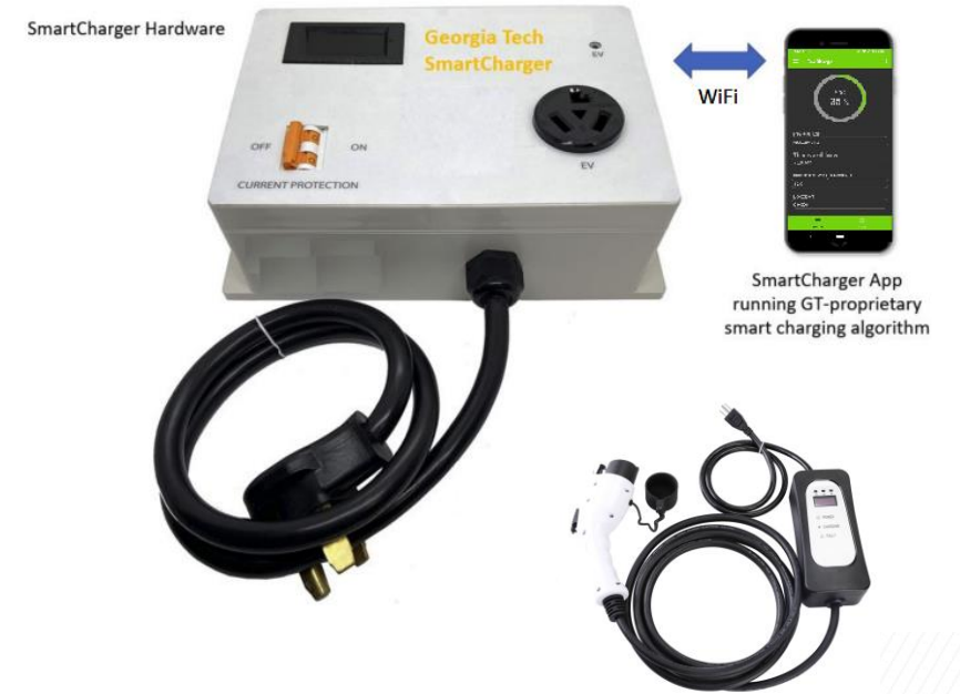
EV charging cable plugs into receptacle in smart charger
